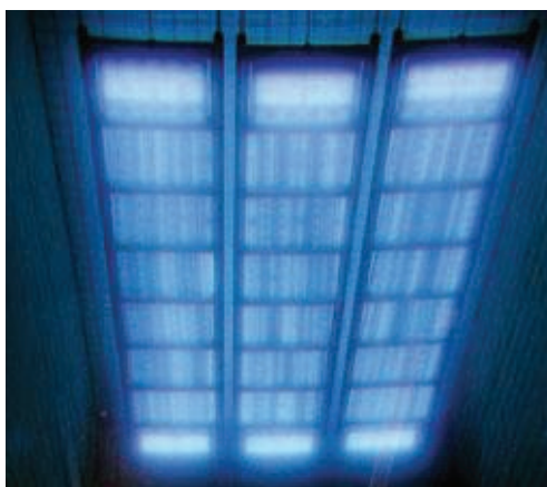
Figure 1. Gamma rays are generated from Cobalt-60 sources. Photo courtesy of STERIS Isomedix Services.
