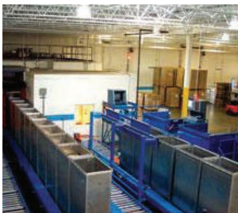
Figure 2. Totes entering an irradiation chamber according to a predetermined loading pattern. Photo courtesy of STERIS Isomedix Services.
