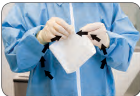
(4) Refold the wiper as shown in Step 2 to enclose the two contaminated faces and expose the two clean faces. Repeat Step 3 using the two clean faces.
