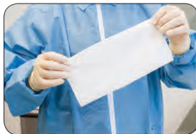
(5) Wiper may be completely unfolded, reversed, and refolded beginning again at Step 1 to enclose the four remaining clean faces.
