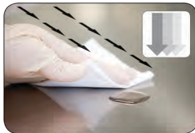
(3) Work from the cleanest areas to the dirtiest areas in long, overlapping unidirectional strokes. Each face of the wiper will be used for one straight stroke. Turn the wiper over and make a second stroke.
